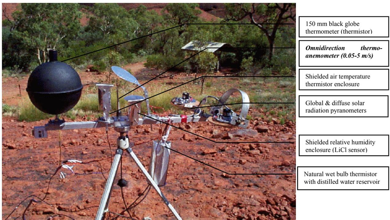
**Fig. 7** The tripod with sensors measuring all relevant heat balance variables as well as *WBGT* parameters.
